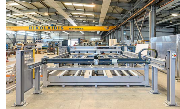
Heavy Duty lifting table platform: In standalone frame to avoid vibrations on machine's stability. Moving on 4 large trapezoidal screws. Maximum lifting capacity 600mm.
