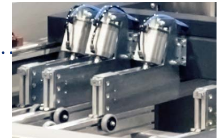
Powerful pusher for panel movement Gripper's projection 100mm Rack-pinion pusher travel system Sliding on high quality round linear guides Max accuracy up on double measuring system: thanks to magnetic tape and servo.
