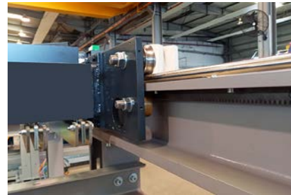
Heavy duty (H) beams pusher movement by rack - pinion system (Atlanta). Smooth movement without vibrations.
